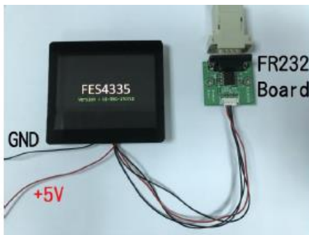
Option2. (RS232 connectivity w/ FR-DCE board)
