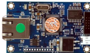
Option3. (LAN connectivity w/ FR-E2S board)
